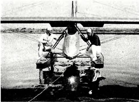
Franklin Woolcott, left, and Don Stevens inspect their stunting pontoon-equipped glider. It is launched by towing it with a fast boat or airplane. It can be looped and rolled.
