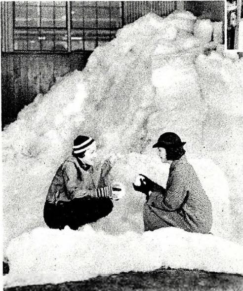
This is not snow but glass, the same kind from which bottles are made. One pound of this substance contains enough fibres to reach around the world. Each strand is 1/20th the diameter of a hair; 100 are needed to make No. 50 thread.
