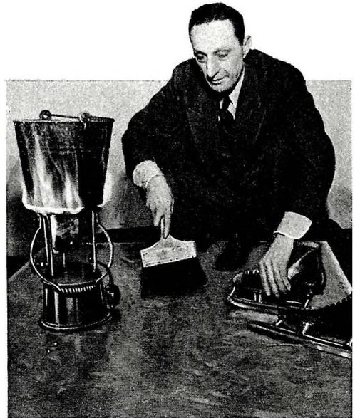
Applied to any surface in boiling liquid form this chemical ice hardens in a few hours leaving a skating rink equal to one of actual ice. The chemical may be reheated and used again.
