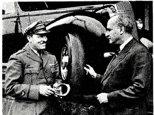
Col. Roscoe Turner, famous speed flier, is shown here examining the latest type of tire tread. The thin rubber vanes of this tire form a serpentine tread when brakes are applied.
