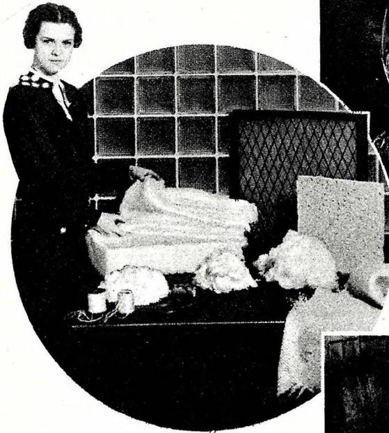
Few would guess that the fluffy batting held by the young lady was made of glass. But it was, and so were the spools of yarn, the woven mat, the bundles and block of insulating material and the screened air filter. Even the wall is made of glass.
